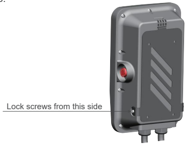
Charger box locking on back plate diagram
