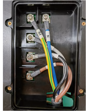
Cable harness diagram FEV-T16/32 (3Ph Connection guide)
